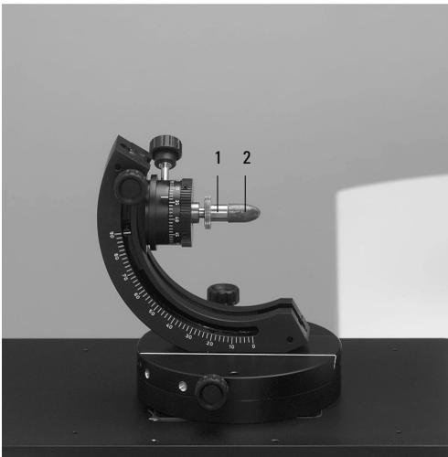
**Fig. 39** Adjustable holder with receptacle for deformed bullets
