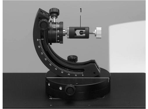
**Fig. 45** Adjustable holder with receptacle for locking cylinders
